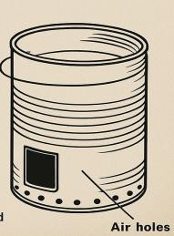
A hobo stove is a simple, lightweight, and efficient wood-burning stove made from a tin can. Perfect for camping or survival use. This guide shows how to build one safely using basic tools and scrap materials. Follow the steps and diagram for a reliable outdoor cooking option.
